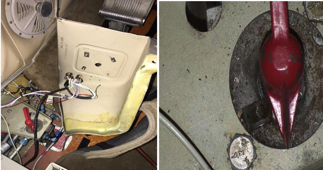
(photo 1) Interior/fuel selector cover removed.
