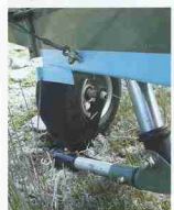
The broken tailwheel before the field repair.
