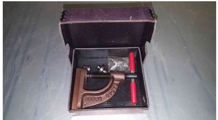
Brake pad riveting tool
